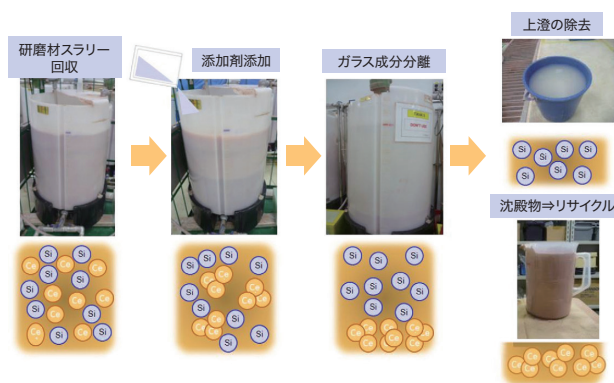
Fig. 8 Conceptual diagram of recycle of cerium oxide polishing slurry by addition agent.
